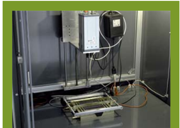
▲ The experimental setup for electroluminescence measurements. The cell is placed underneath the camera and electrically contacted from both sides.
